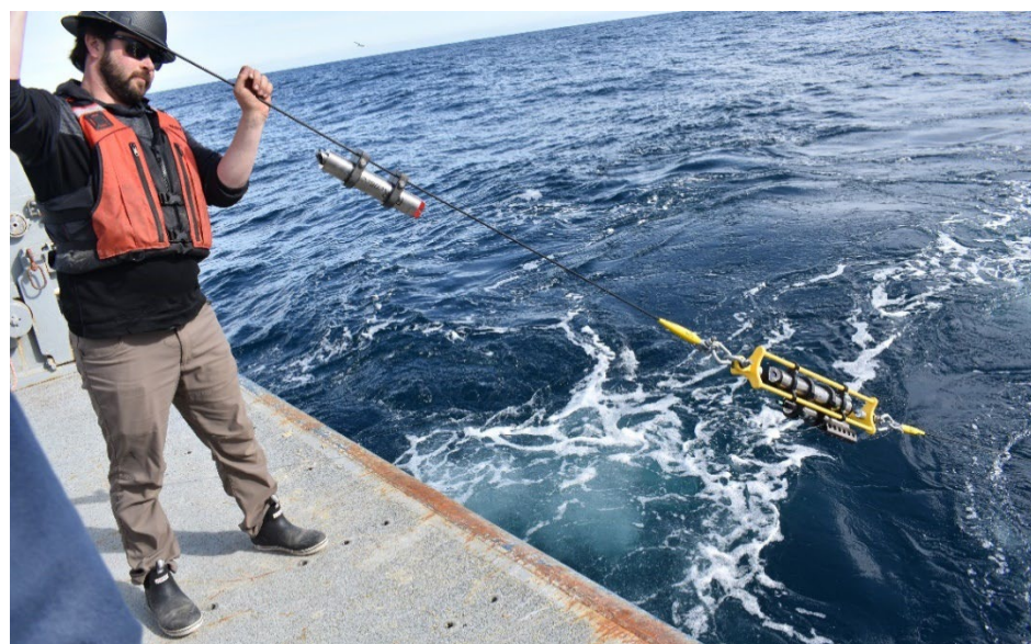
Photo: Chris Basque guides instuments over the transom. Photo shows distance between current meter/microcat and optode, when optode placed lower on wire. This configuration was on all but one instrument sets on moorings M1, M2, and M3.
