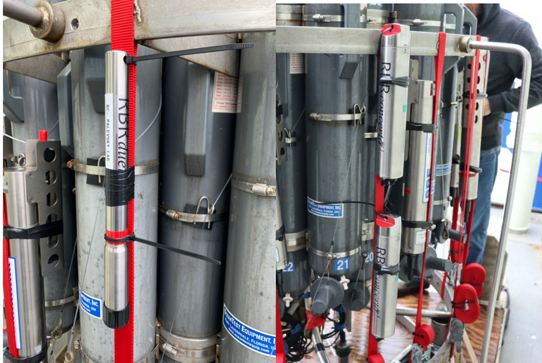
Figure H38. RBR optode Duette (left, photo by E. Park) and Concerto (right, photo by H. Furey) and setup for calibration dips
